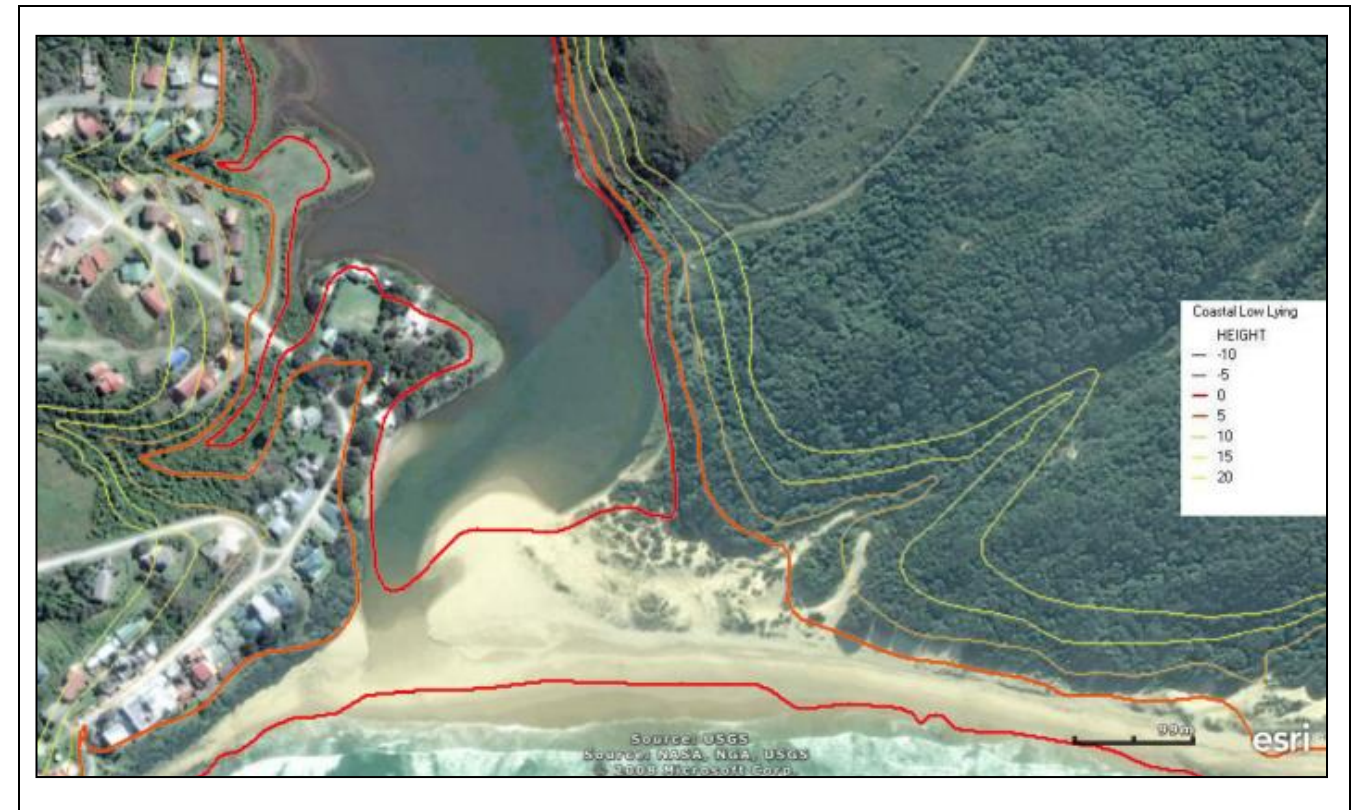
FIGURE NO. 12: THE MORGAN BAY CONTOUR MAP SHOWING SIGNIFICANT INUNDATION OF THE 5M CONTOUR BY PROJECTED SEA LEVEL RISES.
